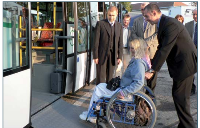
Prostejov's low-platform Ecobuses with ascending ramps are particularly appreciated by paraplegics and mothers with prams. They also have acoustic signal devices helping vision-impaired people to find their way more easily. Last but not least, each Ecobus produces 8,200 kg less of pollutants per year compared to a regular bus – which is appreciated by everyone.
